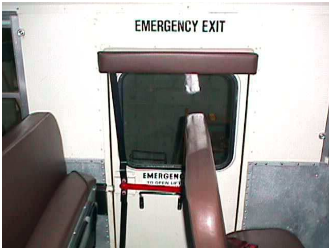
Figure 5. View of side emergency door and “flip-up bottom” seat in the up position.
