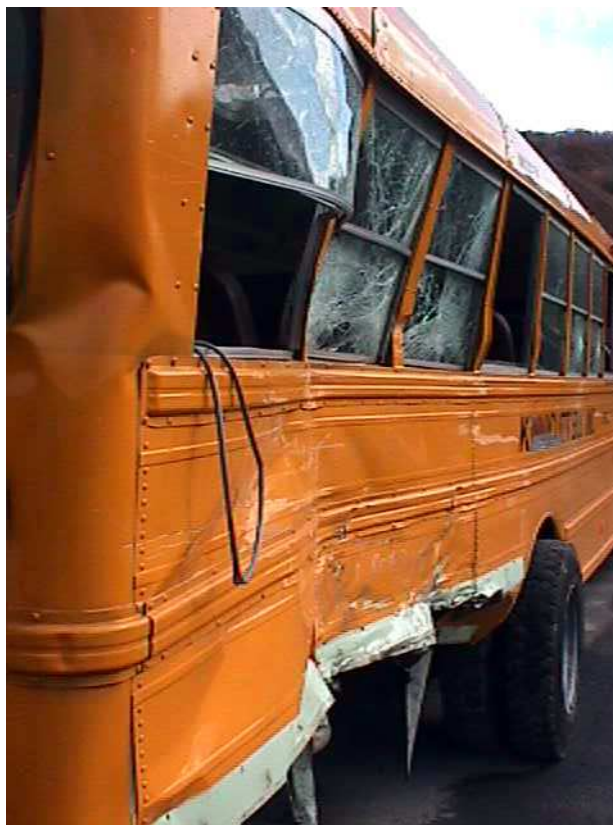
Figure 1. Exterior crush damage of school bus.
