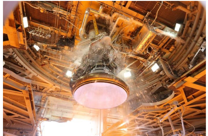
Pictured Above: J-2X Engine Test
