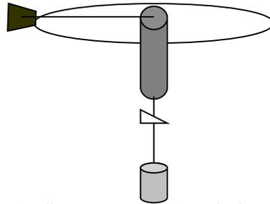
If no net force acts on a moving object, it will continue in a straight line. To cause an object to travel in a circular path, a force must constantly act perpendicular to the direction of motion forcing it inward. This force, called the **centripetal force**, will therefore always be directed toward the center of the circle.
